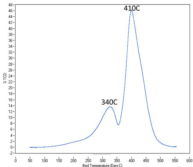
From the analysis graph two clearly defined, but overlapping, peaks are displayed. The first peak has a maximum temperature of 340C. The second peak's maximum is at 410C. However, it should be noted that the peak position can vary depending on the exact placement of the bed thermocouple and the exact composition of the H2-Ar mixture.
