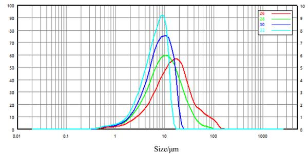
**Figure 4.** Particle size distribution of non-micronized sample under different pressures: red, green, navy, and cyan curve respectively represent 0.1, 0.2, 0.3, and 0.4 Mpa
