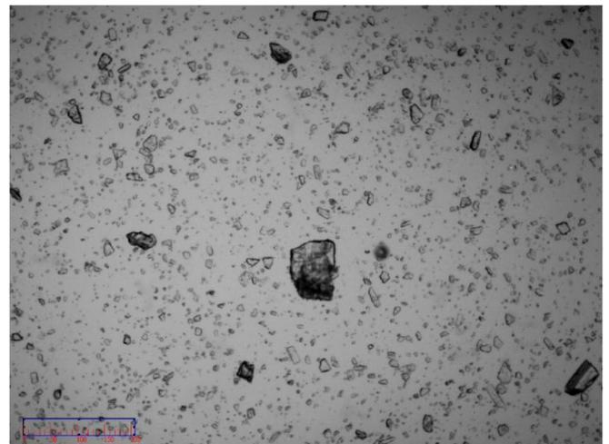
**Figure 5.** Image of non-micronized particles
