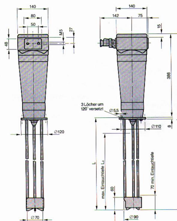
Standard lengths for the measuring system are: 20, 30 and 50 cm. Depending on usage, lengths of up to 130 cm can be commissioned.
