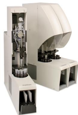
Biotage offers a complete range of sample preparation consumables and instruments including the RapidTrace SPE Workstation. The RapidTrace is a modular, highly scalable and automated sample preparation platform designed for automated processing of 1 mL, 3 mL and 6 mL cartridges.
