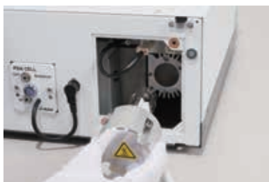
Front panel access for easy lamp replacement
