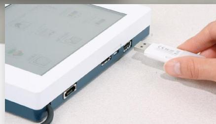
**Spectra Analysis software for PC included as standard** - Data acquired using the iRM can be transferred and analyzed using Spectra Analysis on a PC.
