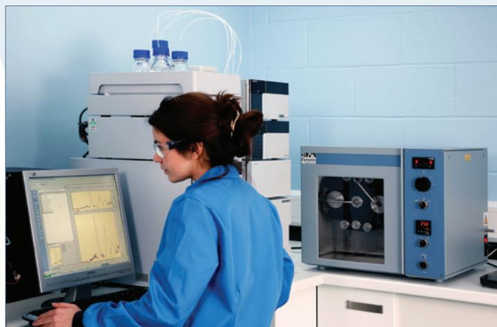
HPLC systems are configurable with one or more typical liquid chromatography detectors including UV, ELSD and MS enabling detection and potential identification of the widest possible range of compounds. Options regarding autosampling and fraction collection are also offered. With these options, Dynamic Extractions can provide systems to suit a wide range of applications and fit all budgetary scales.
