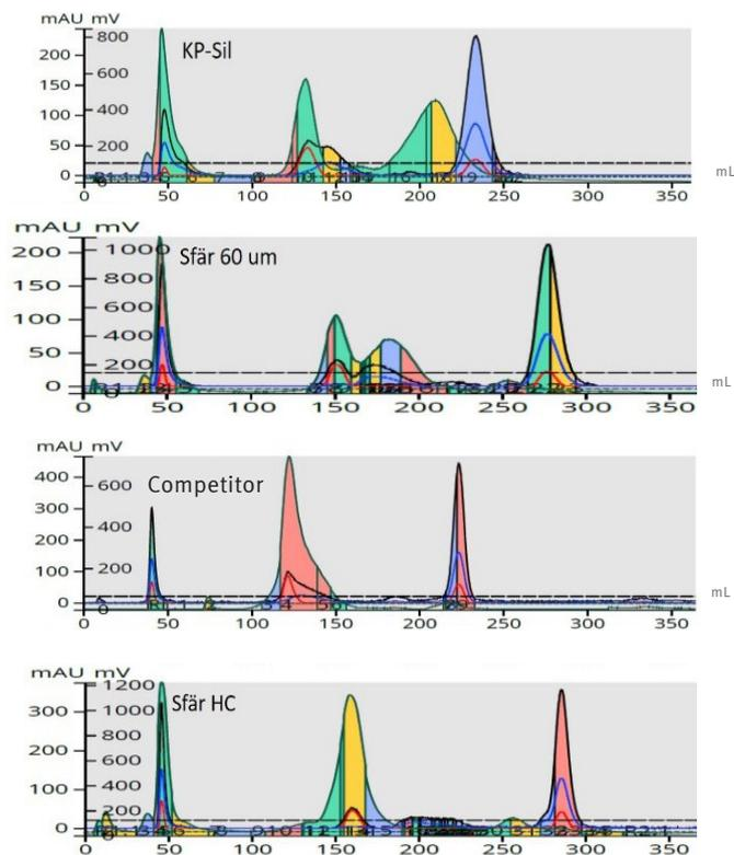
**Figure 4.** Column comparison of a natural product extract using both diode array UV and ELSD for fractionation.**Results:**
