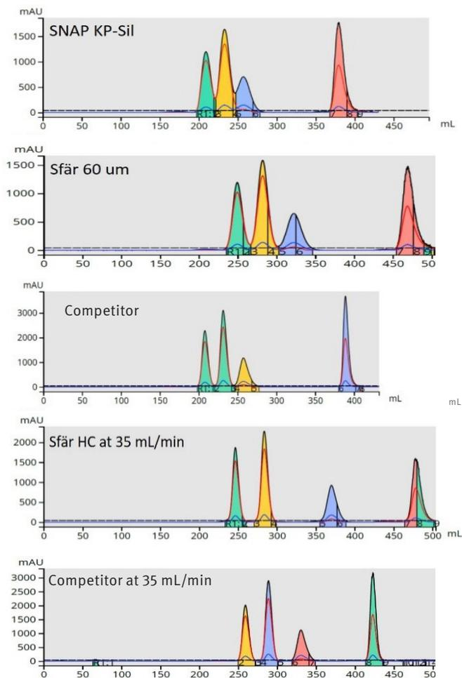
**Figure 2.** Column performance comparison with a 4-component mix.
