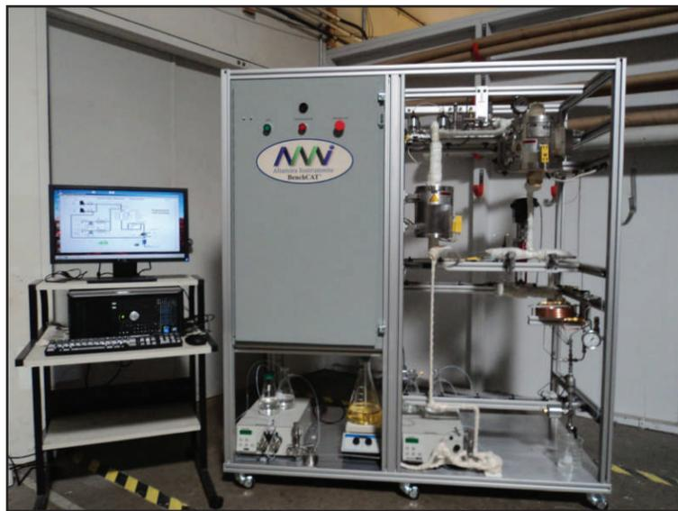
Figure 4. BenchCAT reactor for supercritical trans-esterification of lipids.
