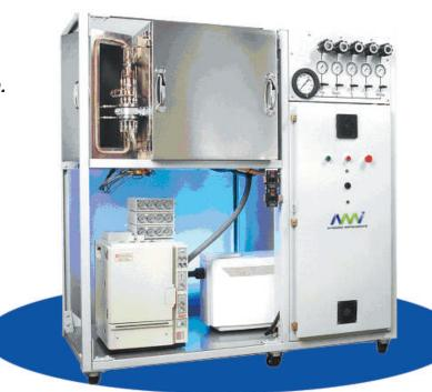
reactor tubes using a set of matched capillaries. A single closure is required to seal all eight reactors. The reactor effluents are routed through heated lines to a condenser and a multiposition selector valve. Analysis of the products is accomplished by gas chromatography. The unit was designed to hold up to 10 mL of catalyst in each reactor and operate at 650 °C and 800 psig.
