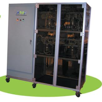
up to 600°C and 30 atmospheres, respectively. All reactor effluents are routed through heated lines to a heated multiposition valve for sequential sampling into a mass spectrometer. Lexan covers are provided for added safety.
